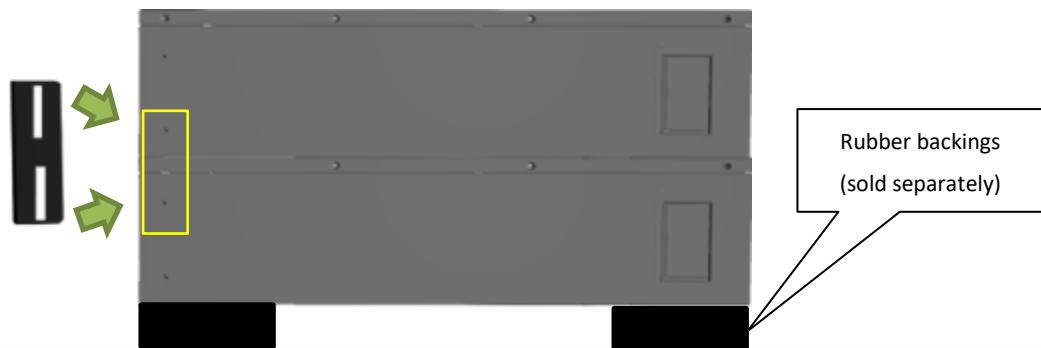
Step 4: Once each battery has been installed horizontally, the feet supplied with the battery in standard configuration can be removed and installed through the modules to constrain the modules on both sides.
