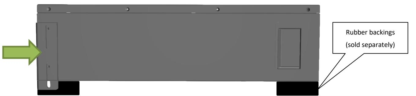
Step 3.a: Lift and place the second battery on top of the first already installed on the floor on its rubber feet.
