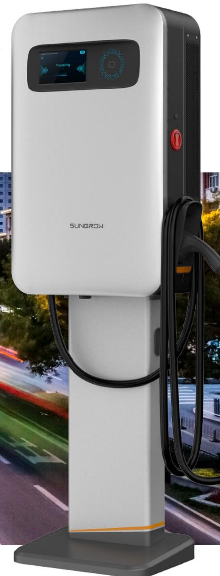
Our 30 kW DC charger is able to **charge EV batteries between 200 to 1000 V<sub>DC</sub>** which covers all the EV car brands to date. Its maximum output current is 80 A. It can resist harsh outdoor conditions such as wet, dusty and salty environments thanks to its IP 65 rating. The electrical emissions are suitable for residential purposes (EMC Class B).
