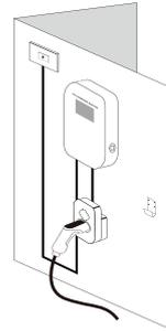
Insert the plug into socket
